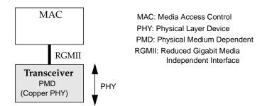
FIGURE 28-5 Transceiver's Role in 1G copper Ethernet
