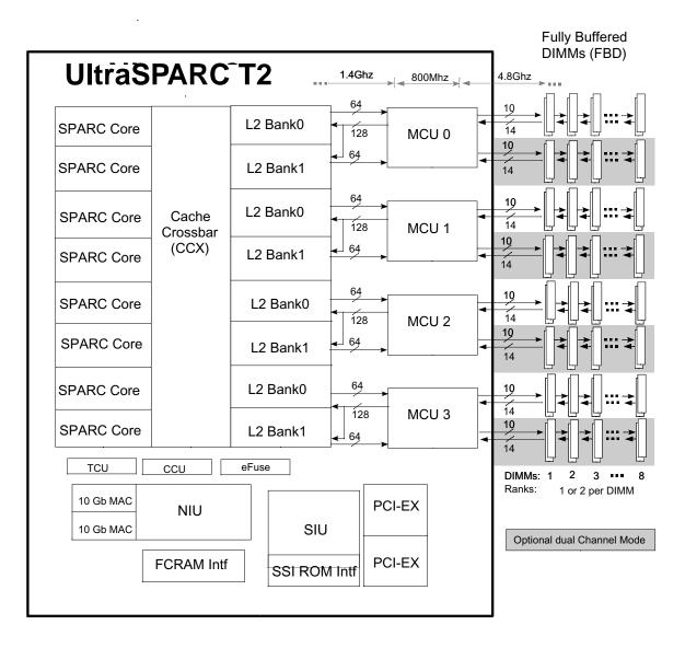
FIGURE 1-2 UltraSPARC T2 Chip Block Diagram
