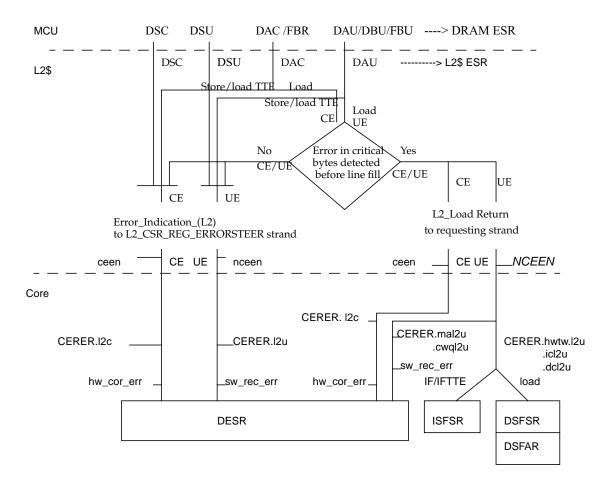
FIGURE 16-2 DRAM Error Flow From MCU to L2 Cache
