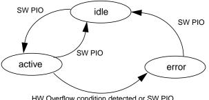
HW Overflow condition detected or SW PIO
