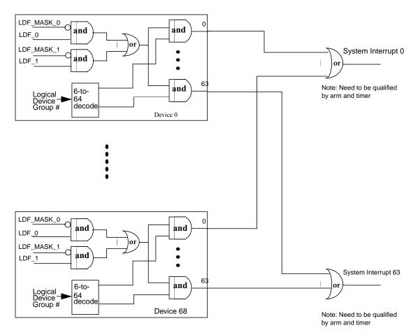
FIGURE 23-1 Interrupt Muxing Logic
