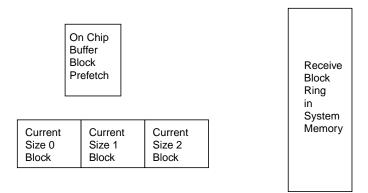
FIGURE 25-1 Buffer Block Ring
