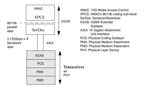
FIGURE 28-3 Transceiver's Role in 10G Ethernet
