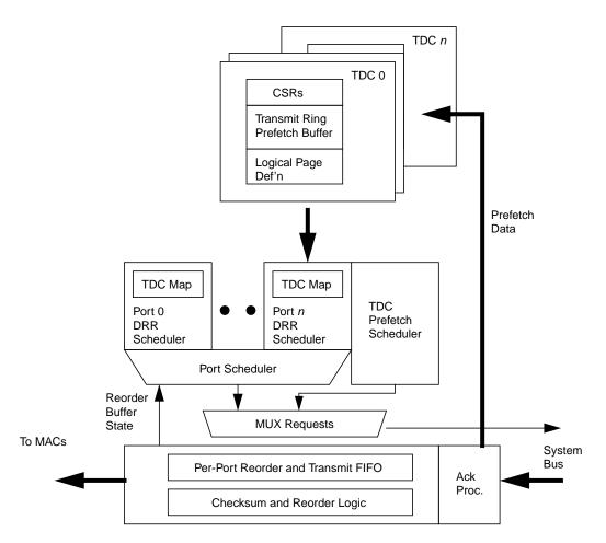
FIGURE 22-5 Transmit Functional Blocks
