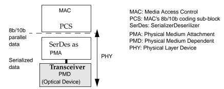
FIGURE 28-4 Transceiver's Role in 1G Fiber Ethernet
