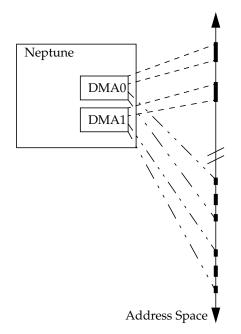
PIOs, controlled accesses via virtualization addresses. This is typicalled enforced by the MMU of the processor.
