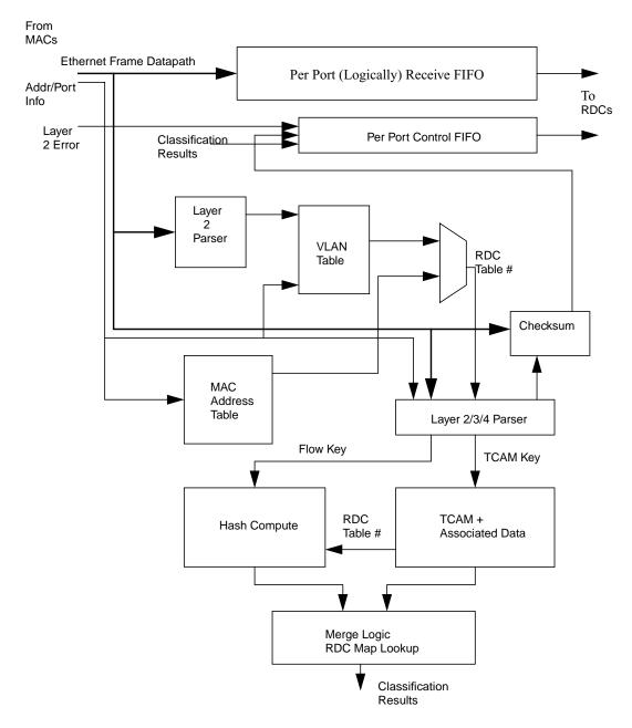
FIGURE 22-3 Receive Buffer and Classification Logic
