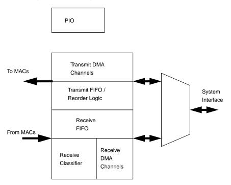
FIGURE 22-1 Ethernet Network I/O Subsystem Architecture
