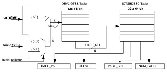
FIGURE 21-2 Reading IOTSB descriptor for a request
