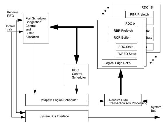
FIGURE 22-4 Receive DMA Channels
