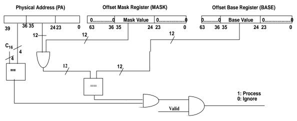
Process = (pa{39:36} = C<sub>16</sub>) and ((PA{35:24} and mask) = base)) and Valid
