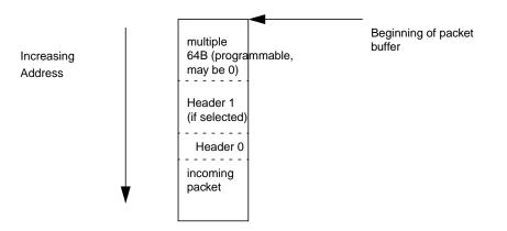
FIGURE 24-1 Packet Buffer Layout
